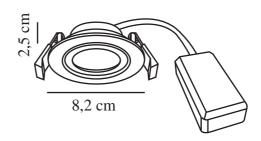
Tension (V): 220-240 Volt Protection IP: IP20 Classe (Classe 1, Classe 2, Classe 3): Classe 2 (Double isolation)
