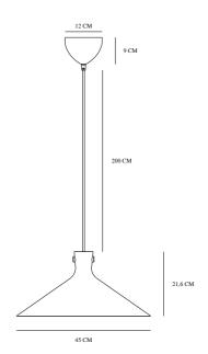
Voltage (V): 220-240 Volt IP degree: IP20 Maximum bulb wattage (W): 60W Class (Class 1, Class 2, Class 3): Class 2 (Double isolated) Socket type: E27 Parallel connection: False
