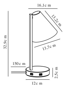
Voltage (V): 220-240 Volt IP degree: IP20
