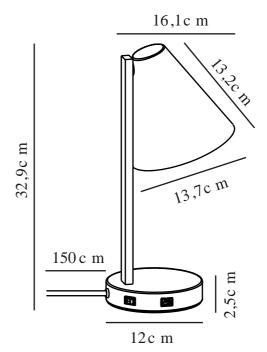
Voltage (V): 220-240 Volt IP degree: IP20 Maximum bulb wattage (W): 40
