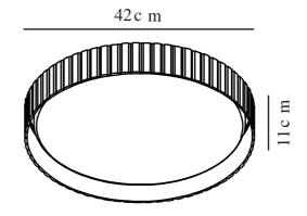
Voltage (V): 220-240 Volt IP degree: IP20 Maximum bulb wattage (W): 3x15W Class (Class 1, Class 2, Class 3): Class 2 (Double isolated) Socket type: E14 Parallel connection: False
