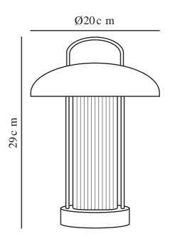
Voltage (V): 3,7 Volt IP degree: IP20 Class (Class 1, Class 2, Class 3): Class 2 (Double isolated) Socket type: LED Module Switch placement: On the fixture Parallel connection: False
