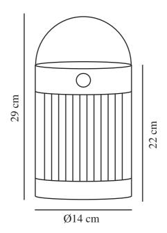
Voltage (V): 5 Volt IP degree: IP44 Class (Class 1, Class 2, Class 3): Class 3 (12V) Socket type: SolarLed Switch placement: On the fixture Parallel connection: False
