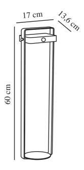
Voltage (V): 5 Volt IP degree: IP44 Class (Class 1, Class 2, Class 3): Class 3 (12V) Socket type: SolarLed Switch placement: On the fixture
