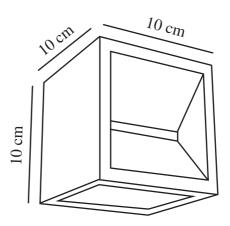
Voltage (V): 220-240 Volt IP degree: IP54
