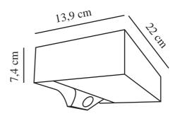
Voltage (V): 5 Volt IP degree: IP44
