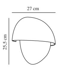
Voltage (V): 220-240 Volt IP degree: IP44 Maximum bulb wattage (W): 25W Class (Class 1, Class 2, Class 3): Class 2 (Double isolated) Socket type: E27 Parallel connection: True
