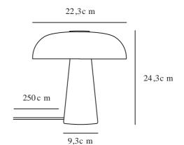
Voltage (V): 220-240 Volt IP degree: IP20 Maximum bulb wattage (W): 15 Class (Class 1, Class 2, Class 3): Class 2 (Double isolated) Socket type: E14 Switch placement: On the cable Parallel connection: False
