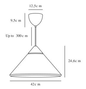
Voltage (V): 220-240 Volt IP degree: IP20 Maximum bulb wattage (W): 60 Class (Class 1, Class 2, Class 3): Class 2 (Double isolated) Socket type: E27 Parallel connection: False
