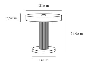
Voltage (V): 3,7 Volt IP degree: IP20 Class (Class 1, Class 2, Class 3): Class 3 (12V) Socket type: LED Module Switch placement: On the fixture Parallel connection: False
