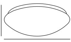
Voltage (V): 230 Volt IP degree: IP44 Class (Class 1, Class 2, Class 3): Class 1 (Earth contact) Socket type: LED - Nonreplaceable light source Parallel connection: True
