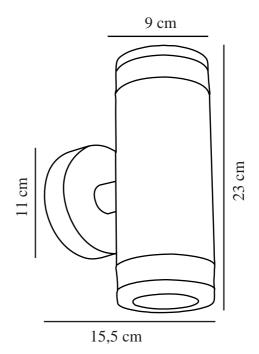
Voltage (V): 230 Volt IP degree: IP44 Maximum bulb wattage (W): 28 Class (Class 1, Class 2, Class 3): Class 1 (Earth contact) Socket type: GU10 Parallel connection: True
