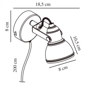
Voltage (V): 220-240 Volt IP degree: IP20
