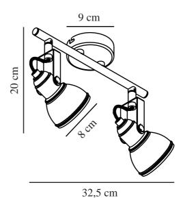
Voltage (V): 220-240 Volt IP degree: IP20 Maximum bulb wattage (W): 35W Class (Class 1, Class 2, Class 3): Class 2 (Double isolated) Socket type: GU10 Dimmerable: Yes with compatible
