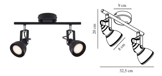
Voltage (V): 220-240 Volt IP degree: IP20 Maximum bulb wattage (W): 35W Class (Class 1, Class 2, Class 3): Class 2 (Double isolated) Socket type: GU10 Dimmerable: Yes with compatible bulb
