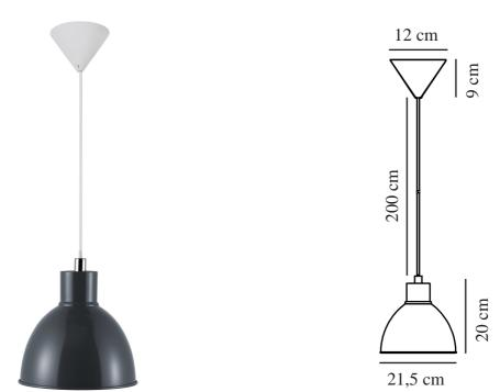
Voltage (V): 220-240 Volt IP degree: IP20 Maximum bulb wattage (W): 40 Class (Class 1, Class 2, Class 3): Class 2 (Double isolated) Socket type: E27 Dimmerable: Yes with compatible bulb Parallel connection: False
