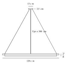
Voltage (V): 230 Volt IP degree if the fixture includes two types of IP degree: IP20 Class (Class I, Class II, Class III): Class 2 (Double isolated) Lampholder type (eg, E27/E14, etc): LED Module Dimmerable: True Switch placement: On the fixture
