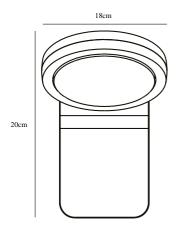
Voltage (V): 230 Volt IP degree: IP44 Class (Class 1, Class 2, Class 3): Class 1 (Earth contact) Bulb base: LED Module Parallel connection: True
