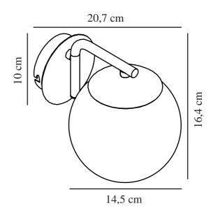
Voltage (V): 230 Volt IP degree: IP20 Maximum bulb wattage (W): 40 Class (Class 1, Class 2, Class 3): Class 2 (Double isolated) Socket type: E14 Dimmerable: Yes with compatible bulb Switch placement: On the cable
