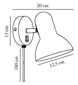
Voltage (V): 230 Volt IP degree: IP20
