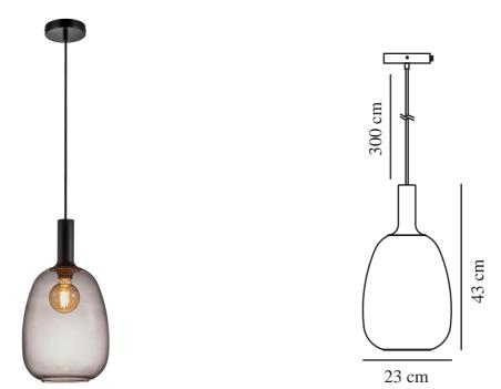
Voltage (V): 220-240 Volt IP degree: IP20 Maximum bulb wattage (W): 60 Class (Class 1, Class 2, Class 3): Class 1 (Earth contact) Socket type: E27 Dimmerable: Yes with compatible bulb
