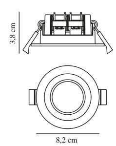
Voltage (V): 230 Volt IP degree: IP20 Class (Class 1, Class 2, Class 3): Class 2 (Double isolated) Socket type: LED - Nonreplaceable light source Parallel connection: True
