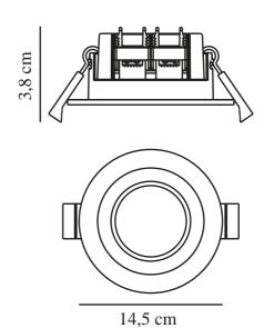
Voltage (V): 220-240 Volt IP degree: IP20 Class (Class 1, Class 2, Class 3): Class 2 (Double isolated) Socket type: LED Module Parallel connection: True
