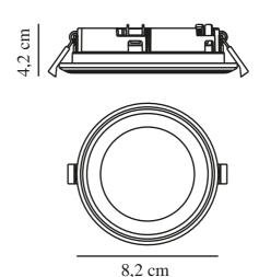
Voltage (V): 230 Volt IP degree: IP20 Class (Class 1, Class 2, Class 3): Class 2 (Double isolated) Socket type: LED – Nonreplaceable light source Parallel connection: True
