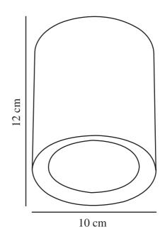
Voltage (V): 230 Volt IP degree: IP20 Class (Class 1, Class 2, Class 3): Class 2 (Double isolated) Socket type: LED Module Parallel connection: True
