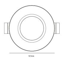
Voltage (V): 230 Volt IP degree if the fixture includes two types of IP degree: IP65 Class (Class I, Class II): Class 2 (Double isolated) Lampholder type (eg, E27/E14, etc): LED Module Parallel connection possible?: True
