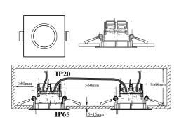
Voltage (V): 230 Volt IP degree if the fixture includes two types of IP degree: IP65 Class (Class I, Class II, Class III): Class 2 (Double isolated) Lampholder type (eg, E27/E14, etc): LED Module Parallel connection possible?: True
