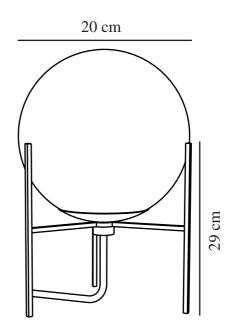
Voltage (V): 220-240 Volt IP degree: IP20 Maximum bulb wattage (W): 15 Class (Class 1, Class 2, Class 3): Class 2 (Double isolated) Socket type: E14 Dimmerable: Yes with compatible bulb Switch placement: On the cable
