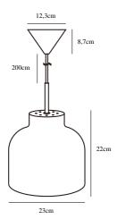
Voltage (V): 230 Volt IP degree if the fixture includes two types of IP degree: IP20 Maximum compatible bulb wattage (W): 25W Class (Class I, Class II, Class III): Class 2 (Double isolated) Lampholder type (eg, E27/E14, etc): E27 Dimmerable: Yes with compatible
