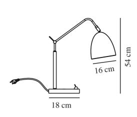
Voltage (V): 220-240 Volt IP degree: IP20
