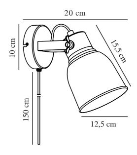
Voltage (V): 220-240 Volt IP degree: IP20
