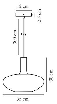
Voltage (V): 220-240 Volt IP degree: IP20
