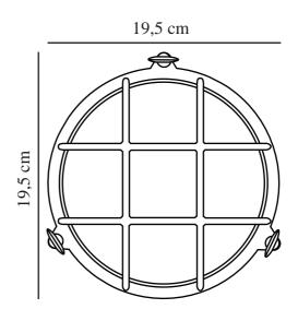
IP degree: IP64 Maximum bulb wattage (W): 12.5 Class (Class 1, Class 2, Class 3): Class 1 (Earth contact)
