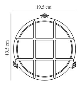
Voltage (V): 230 Volt IP degree: IP64 Maximum bulb wattage (W): 12,5W
