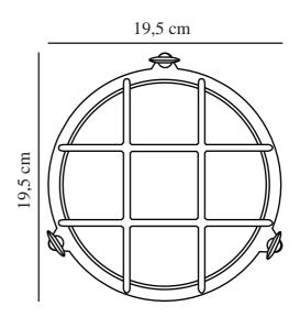
IP degree: IP64 Maximum bulb wattage (W): 12.5 Class (Class 1, Class 2, Class 3): Class 1 (Earth contact)
