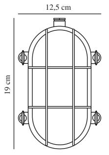
Voltage (V): 230 Volt IP degree: IP64 Maximum bulb wattage (W): 12.5 Class (Class 1, Class 2, Class 3): Class 1 (Earth contact) Socket type: E27 Parallel connection: False
