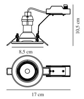
Voltage (V): 220-240 Volt IP degree: IP20 Maximum bulb wattage (W): 35 Class (Class 1, Class 2, Class 3): Class 2 (Double isolated) Socket type: GU10 Dimmerable - Hidden: False Parallel connection: False
