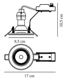
Voltage (V): 220-240 Volt IP degree: IP20 Maximum bulb wattage (W): 35 Class (Class 1, Class 2, Class 3): Class 2 (Double isolated) Socket type: GU10 Dimmerable: False Parallel connection: False
