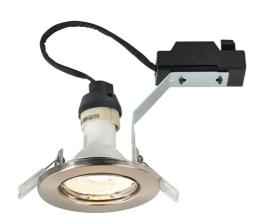
Voltage (V): 220-240 Volt IP degree: IP20 Maximum bulb wattage (W): 35 Class (Class 1, Class 2, Class 3): Class 2 (Double isolated) Socket type: GU10 Dimmerable: False Parallel connection: False
