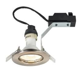
Voltage (V): 220-240 Volt IP degree: IP20 Maximum bulb wattage (W): 50 Class (Class 1, Class 2, Class 3): Class 2 (Double isolated) Socket type: GU10 Parallel connection: False
