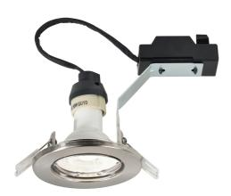
Voltage (V): 220-240 Volt IP degree: IP20 Maximum bulb wattage (W): 50W Class (Class 1, Class 2, Class 3): Class 2 (Double isolated) Socket type: GU10 Parallel connection: False
