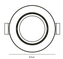
Voltage (V): 230 Volt IP degree if the fixture includes two types of IP degree: IP20 Class (Class I, Class II, Class III): Class 2 (Double isolated) Lampholder type (eg, E27/E14, etc): LED Module Dimmerable: True Parallel connection possible?:
