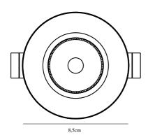
Voltage (V): 230 Volt IP degree if the fixture includes two types of IP degree: IP65 Class (Class I, Class II, Class III): Class 2 (Double isolated) Lampholder type (eg, E27/E14, etc): LED Module Dimmerable: True Parallel connection possible?:
