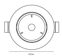
Voltage (V): 230 Volt IP degree if the fixture includes two types of IP degree: IP20 Maximum compatible bulb wattage (W): 50W Class (Class I, Class II, Class III): Class 2 (Double isolated) Lampholder type (eg, E27/E14, etc): GU10 Dimmerable: True Parallel connection possible?:
