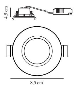
Voltage (V): 230 Volt IP degree: IP65 Class (Class 1, Class 2, Class 3): Class 2 (Double isolated) Socket type: LED Module Parallel connection: True
