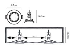
Voltage (V): 230 Volt IP degree if the fixture includes two types of IP degree: IP20 Maximum compatible bulb wattage (W): 50W Class (Class I, Class II, Class III): Class 2 (Double isolated) Lampholder type (eg, E27/E14, etc): GU10 Dimmerable: True
