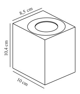
Voltage (V): 230 Volt IP degree: IP44 Class (Class 1, Class 2, Class 3): Class 1 (Earth contact) Socket type: LED – Nonreplaceable light source Dimmerable: False Parallel connection: True
