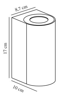
Voltage (V): 230 Volt IP degree: IP44 Maximum bulb wattage (W): 28 Class (Class 1, Class 2, Class 3): Class 1 (Earth contact) Socket type: GU10 Parallel connection: True
